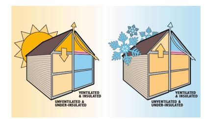
Proper insulation and ventilation minimize the temperature differential between the attic and the air outside, helping reduce energy costs.
